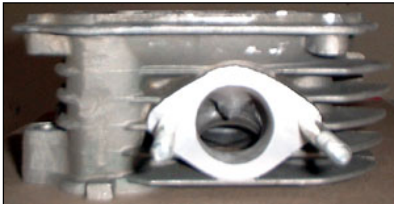
Ported GY6 Engine Intake Port
